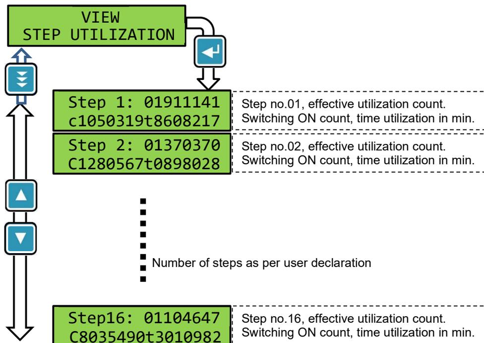
$$\text{COUNTS} = (\text{switching ON counts} / \text{C}) + (\text{ON time in minutes} / \text{T})$$
