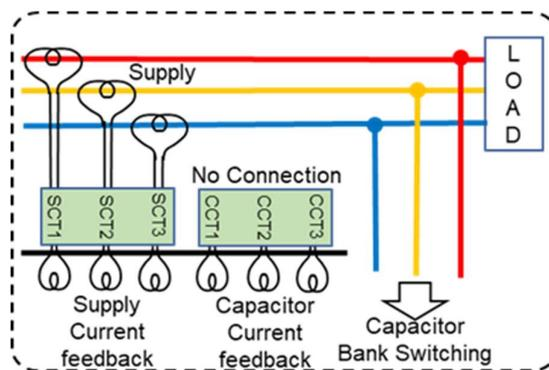
Note: In Cap. Config. No.0, the feedback is from Supply current CTs. This is for Capacitor bank VAR monitoring action.
