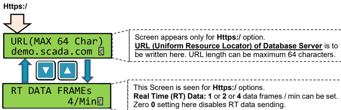
Https:/ communication with GPRS modem connection is the recommended option. The data is transmitted on "Secure" channel. There is a lot of versatility with which the data is transmitted. Data logging has User selectable options for optimal use of the memory.
