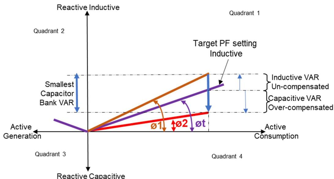
The supply Grid  $PF_1 = \cos(\theta_1)$  when Capacitor Bank is disconnected
