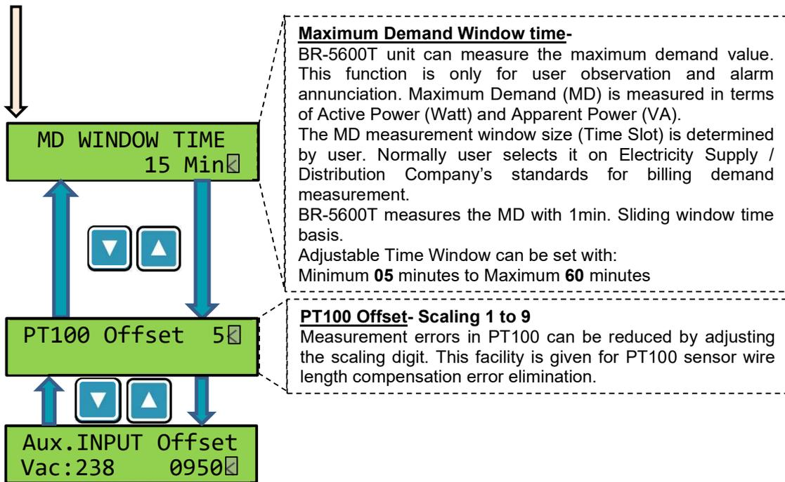
The last Screen in measurement section is for calibration of Auxiliary Input AC voltage measurement. The Calibration settings are to be carried out by user if and only if the Auxiliary input functionality as **CONT-V**. Otherwise, there is no need to carry out any calibration process, and screen would not be available for user to edit.
