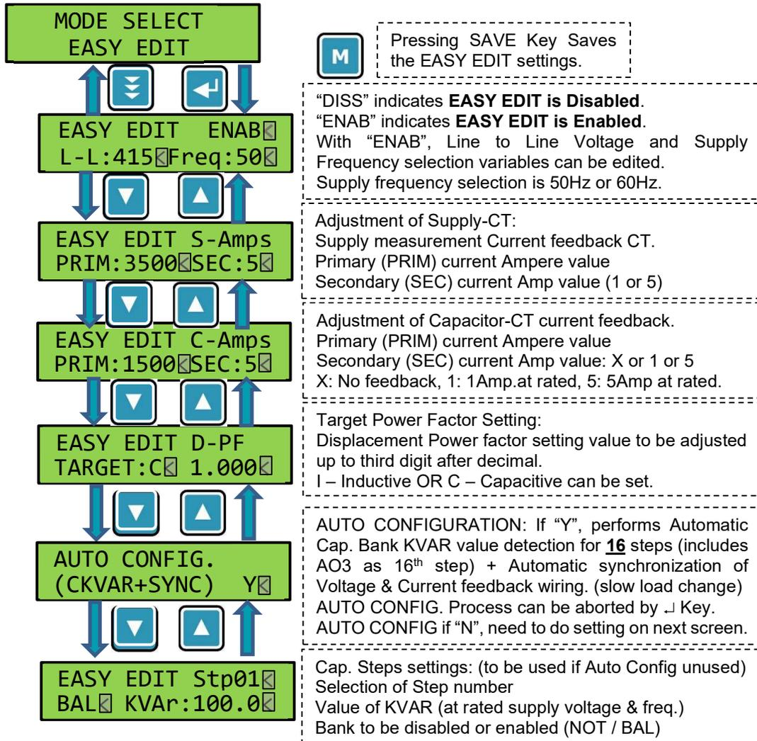
**AUTO COFIGURATION** feature (once enabled) can detect the capacitor bank step KVAR (Reactive Power) value automatically and detects the Voltage & Current feedback wiring. If found wrong, corrects it automatically. This feature prevents the hassles of calculation and is convenient.
