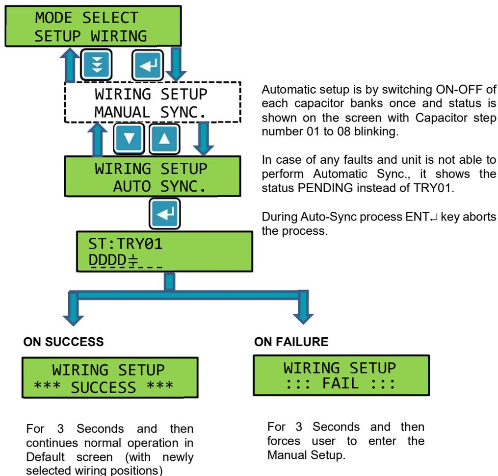
Note that once the Wiring Setup is a Success, the unit BR5600T would remember the success sequence throughout its life. Auxiliary Supply Powering down would not disturb this memorized sequence.
