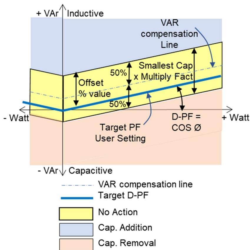
The settings on PFC to adjust the “No Action Band” are:
