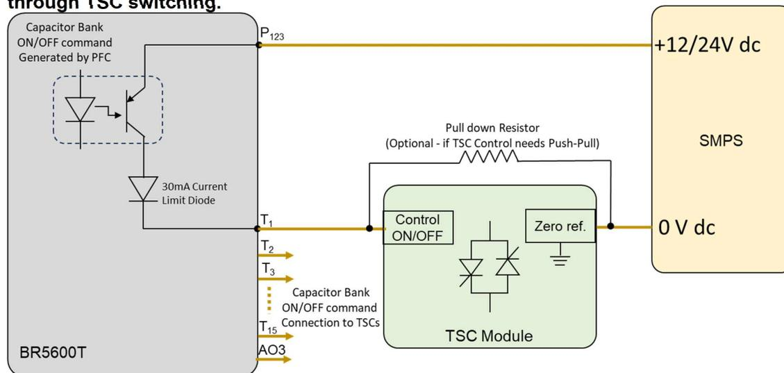
For RTPFC systems, the switching modules are TSC (Thyristor Switched Capacitors) for high-speed turn ON / OFF the capacitors.
